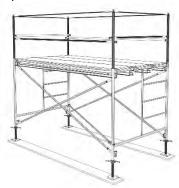
8. Install toe boards as required. The gap between the bottom of the toe board and the top of the platform must not be more than 1/2 inches.
